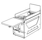
The cooker module contains: two burners, two neoprene-covered gas cartridges, one high drawer for kitchen equipment, one wide drawer for camping utensils, and a bag for small things like spices. It also includes pieces of sheet metal for windproofing that are housed in a practical case.
